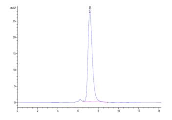
The purity of Biotinylated Human IL-17R alpha is greater than 95% as determined by SEC-HPLC.
